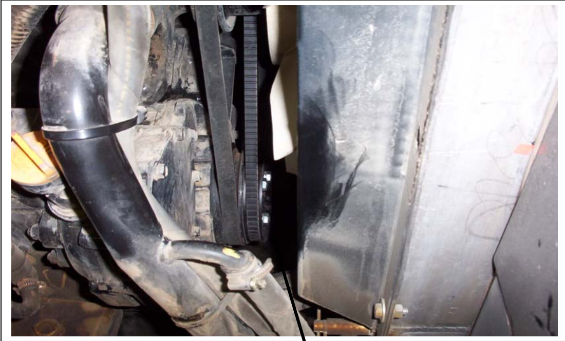
Add on pulley bolted to the crank.
