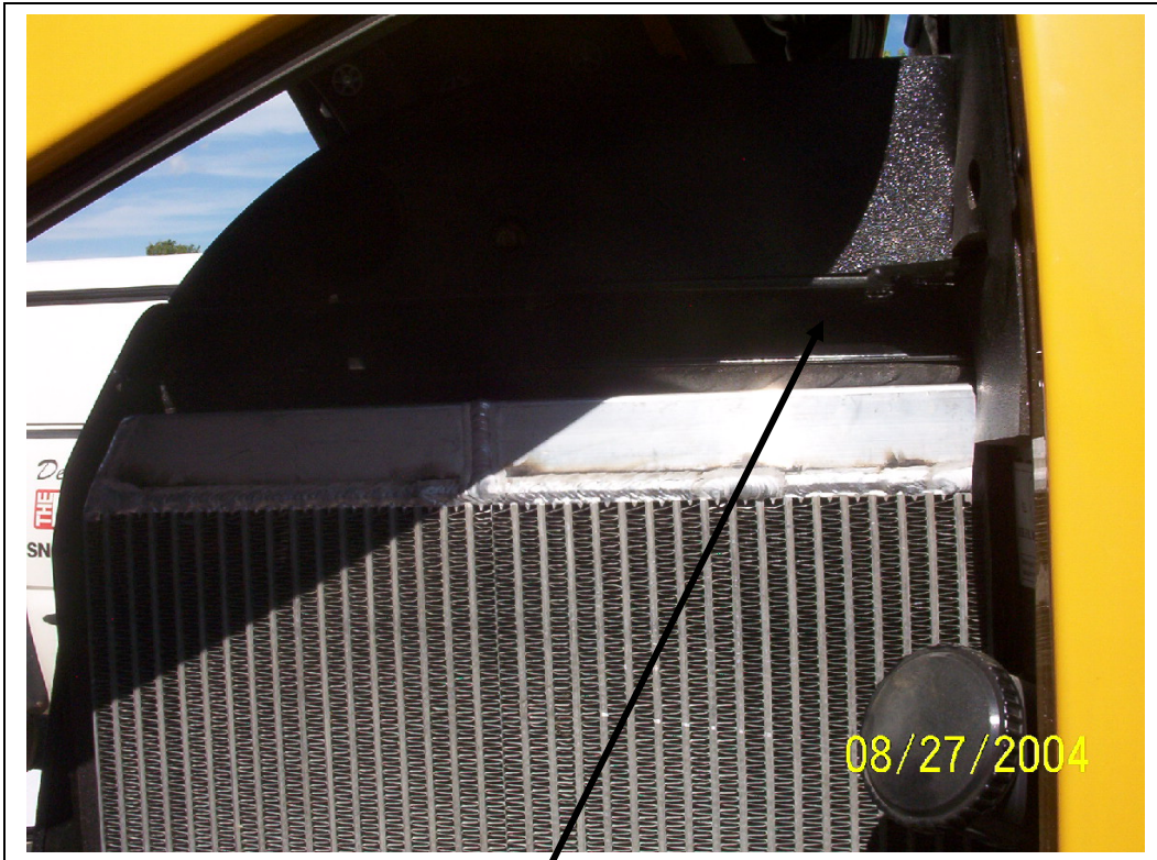
Bolt lower condenser mounts to these bolts.
