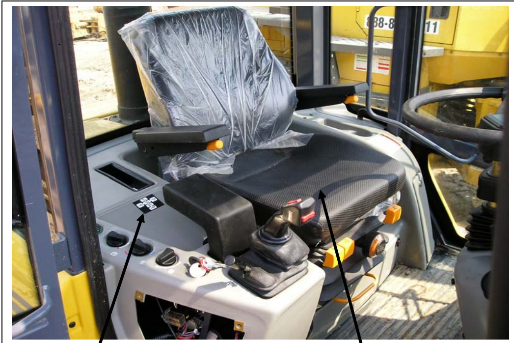
Remove entire plastic housing to install evaporator
